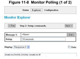
Use Monitor Explorer or directly configure settings in Monitor Poll Configuration. For each message Command, determine an appropriate Timeout and possibly shorten it via a Length and/ or End Character.
